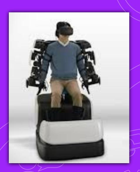
A human operator can controls the robot from Earth, using a VR globes and exoskeleton. Shared Autonomy facilitate time-delayed telepresence
